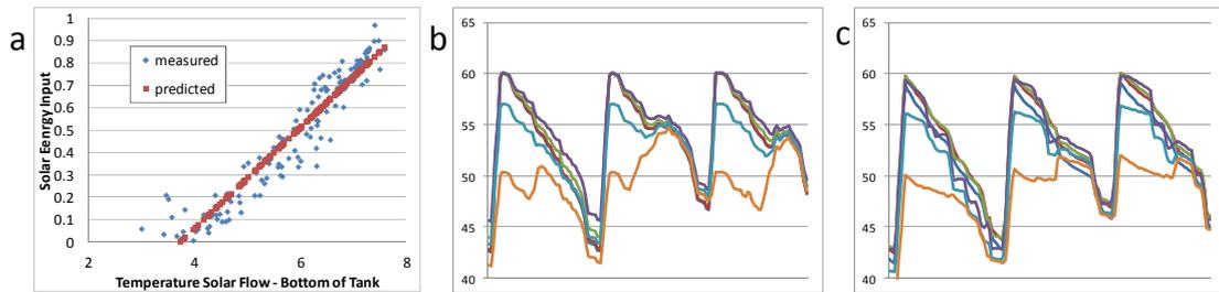
Fig. 6. Model Prediction (a) Solar Energy Regression; (b) Measured Tank Temperatures; (c) Predicted Performance.
